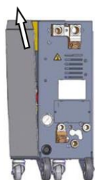
Fig. 87: Extraia a chapa lateral
