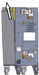
Fig. 91: Pull out the side plate
