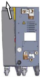
Fig. 91: Pull out the side plate
