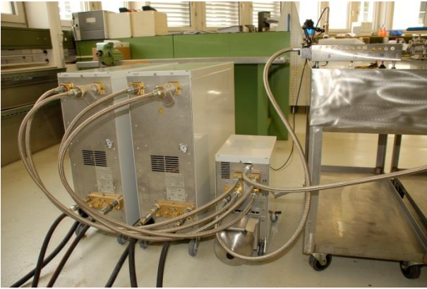
Fig. 1. Example of an installed Vario-5 system (demonstration set-up with test mould and machine simulator)
