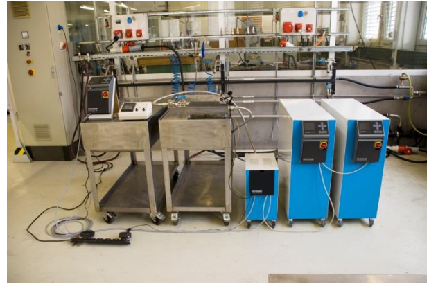
Fig. 1. Example of an installed Vario-5 system (demonstration set-up with test mould and machine simulator)
