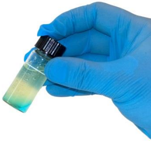
Fig. 16: Shaking and phase separation
