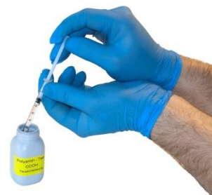
Fig. 14: Fill measurement pipette
