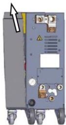
Fig. 71: Pull out the side plate
