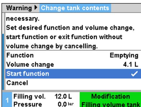
Fig. 30: Turn on Emptying tank contents
