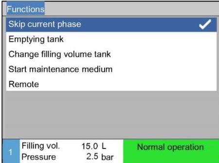
Fig. 27: Enabling Skip current phase
