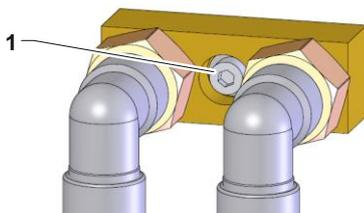
Fig. 10: Central fixing
