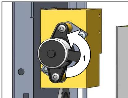
Fig. 75: Remove cooling valve 1
