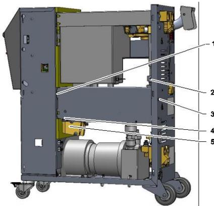
Fig. 74: Removing the heating element
