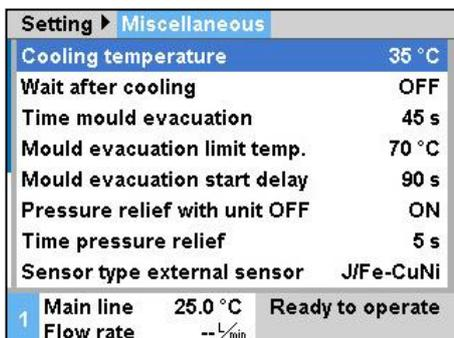
Fig. 41: Cooling temperature
