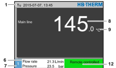
Fig. 21: Basic display Unit operated as module
